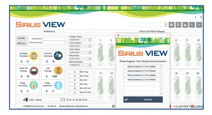
Note: User should enter serial numbers of Modules on rack. This should be done only one time. At execution, application will remember the previous entered serial numbers and user will only need to press register button.
